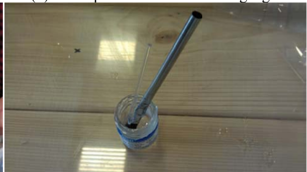
(c) Stir up resin for about 5 minutes and let it set for another 5 minutes
