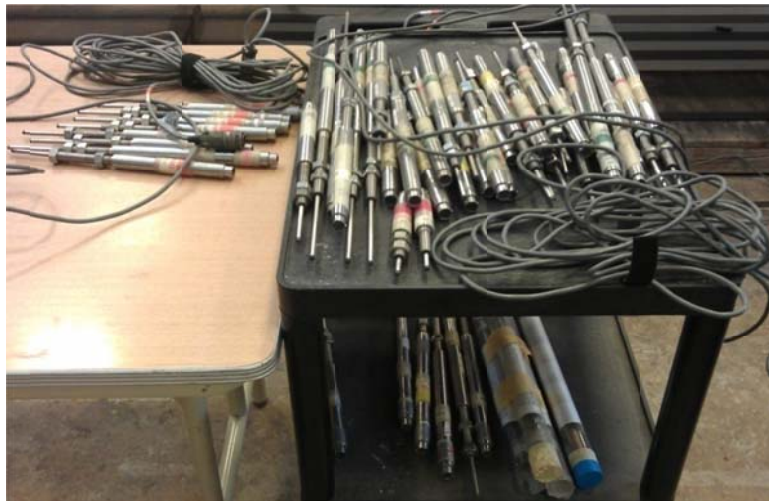
Figure 7.5: DC-LVDTs for box girder tests
