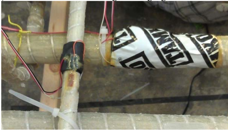
(b) Long-term protection of strain gauges
