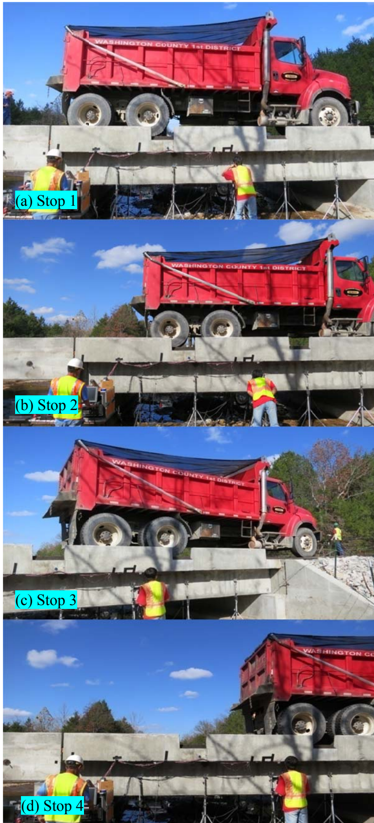
Figure 6.7: Illustrated four steps of one truck over each span
