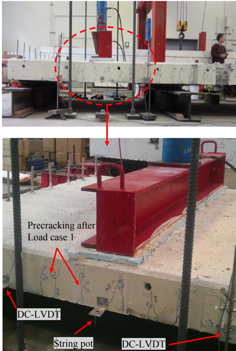
Figure 7.17: Setup for shear test in Load Case 2
