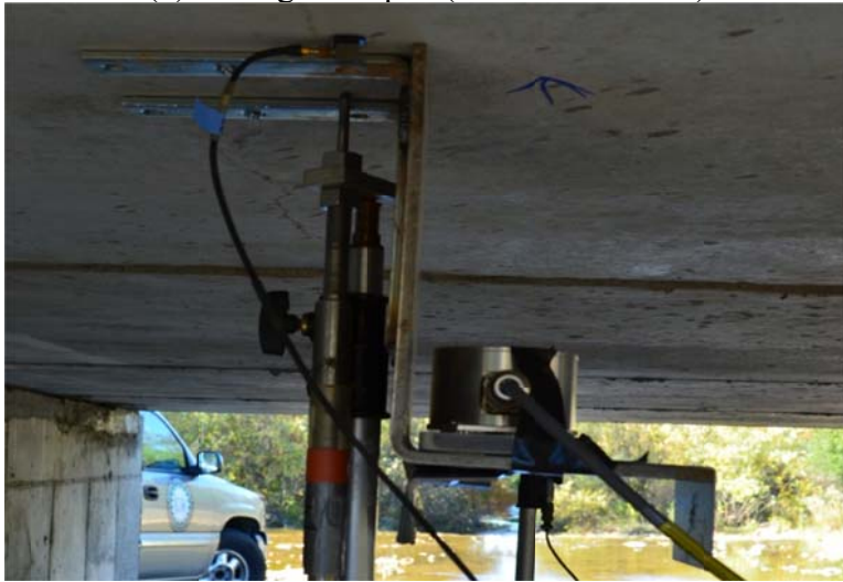
(b) Box girder span (7 accelerometers)
