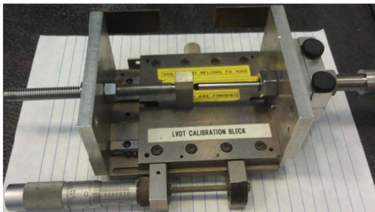
Figure 7.6: Calibration of a DC-LVDT with calibration block
