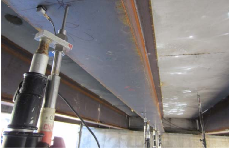
(a) Steel-girder span (7 accelerometers)
