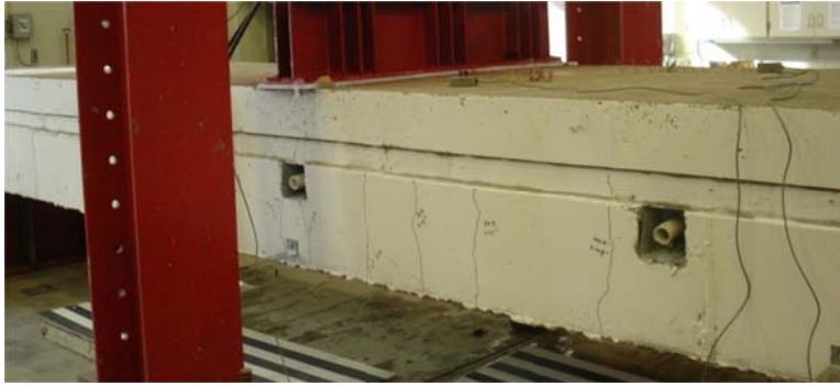
(a) Initial flexural cracks
