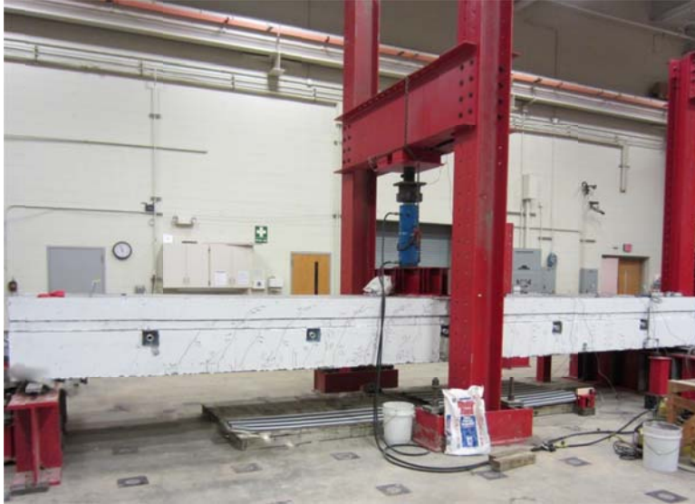
(a) Overview of the crack pattern
