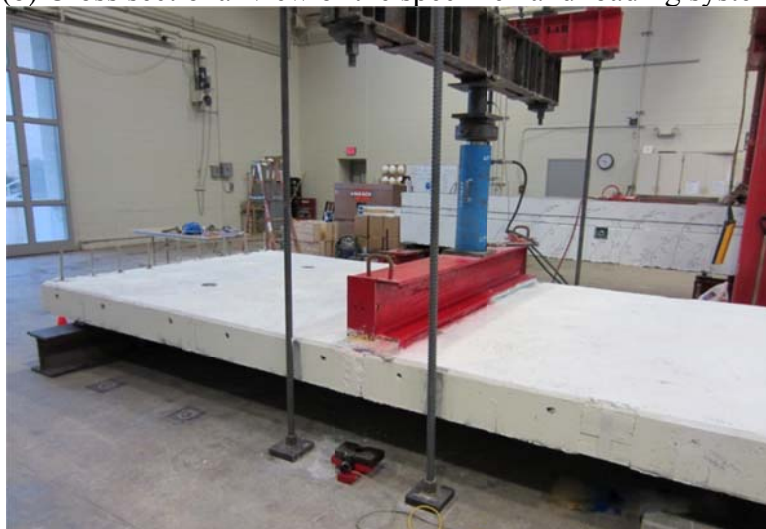
(c) Overview of the loading system
